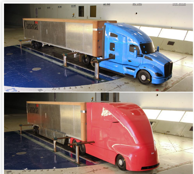
FIGURE 2 Tractor-trailer models: conventional sleeper-cab tractor (top), zero-emission tractor (bottom).
