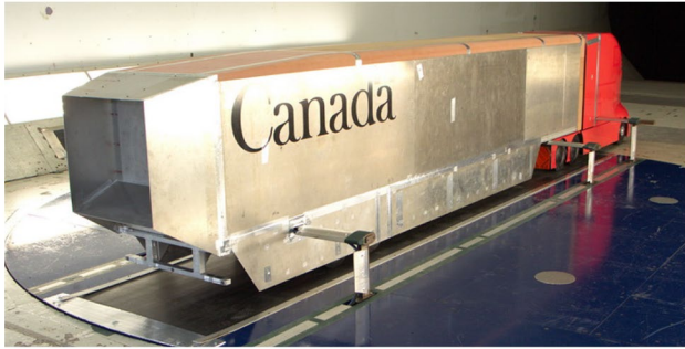
FIGURE 10 Low-drag trailer model with side-skirts, large boat-tail, trailer fairing, and single-wide tires with wheel covers.
