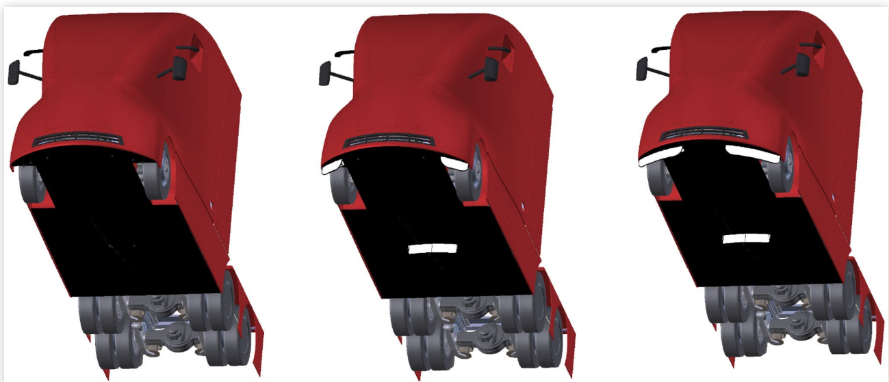
FIGURE 6 Adjustable under-body-panel and air-dam configurations.
