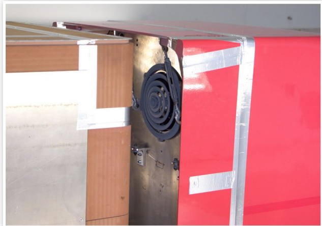
FIGURE 9 Annular diffuser installed over the fan exhaust for the roof-duct cooling flows.
