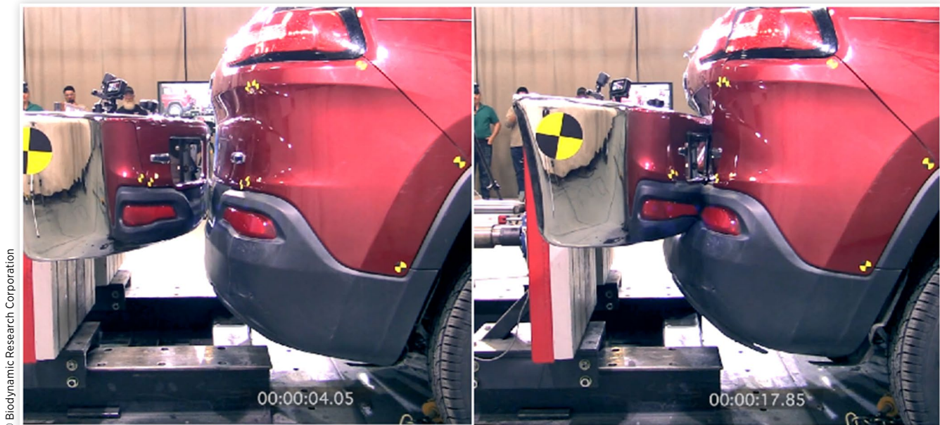
FIGURE 18 Frames from a video of the QSFD measurement for crash test #3. The left frame shows the front bumper of the F-750 front bumper as it contacts the rear of the 2014 Jeep Cherokee, and the right frame shows the bumper near maximum engagement of 0.54 ft (16.5 cm).
