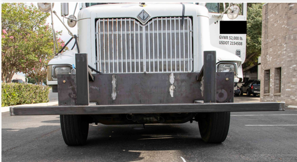
FIGURE 20 An underride guard was mounted on the front of the International 9100 tractor.
