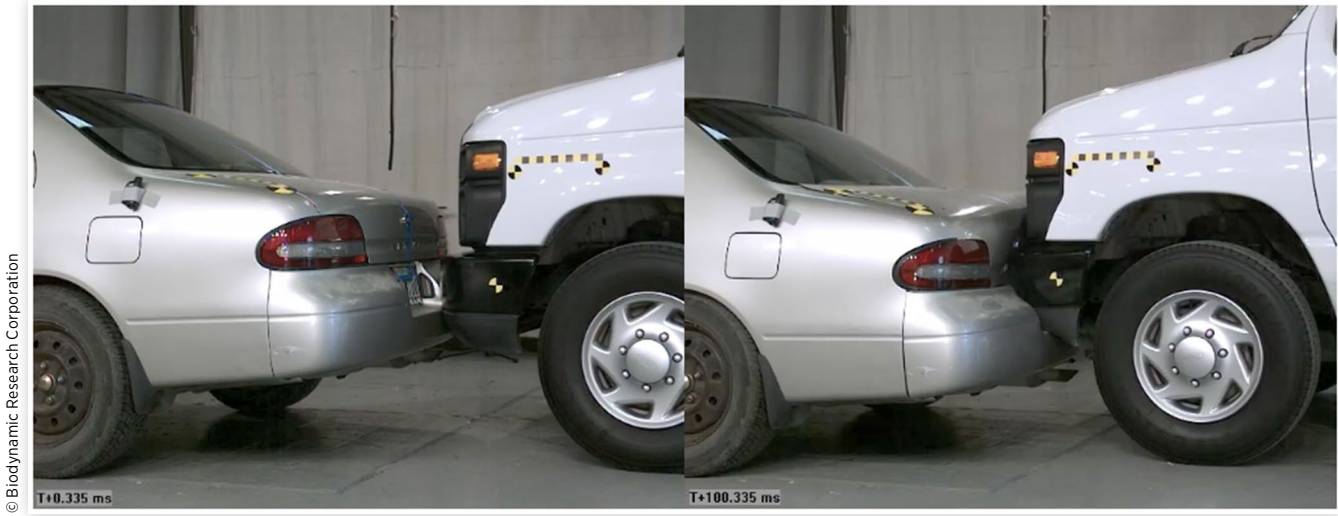
FIGURE 9 The damage to the rear of the 1997 Nissan Altima in crash test #2.
