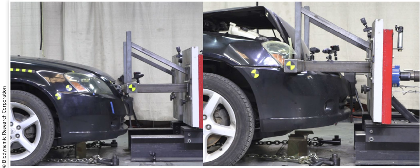
FIGURE 31 Video frames taken during the measurement of the QSF data for crash test #4 show initial contact (left) and maximum engagement (right).
