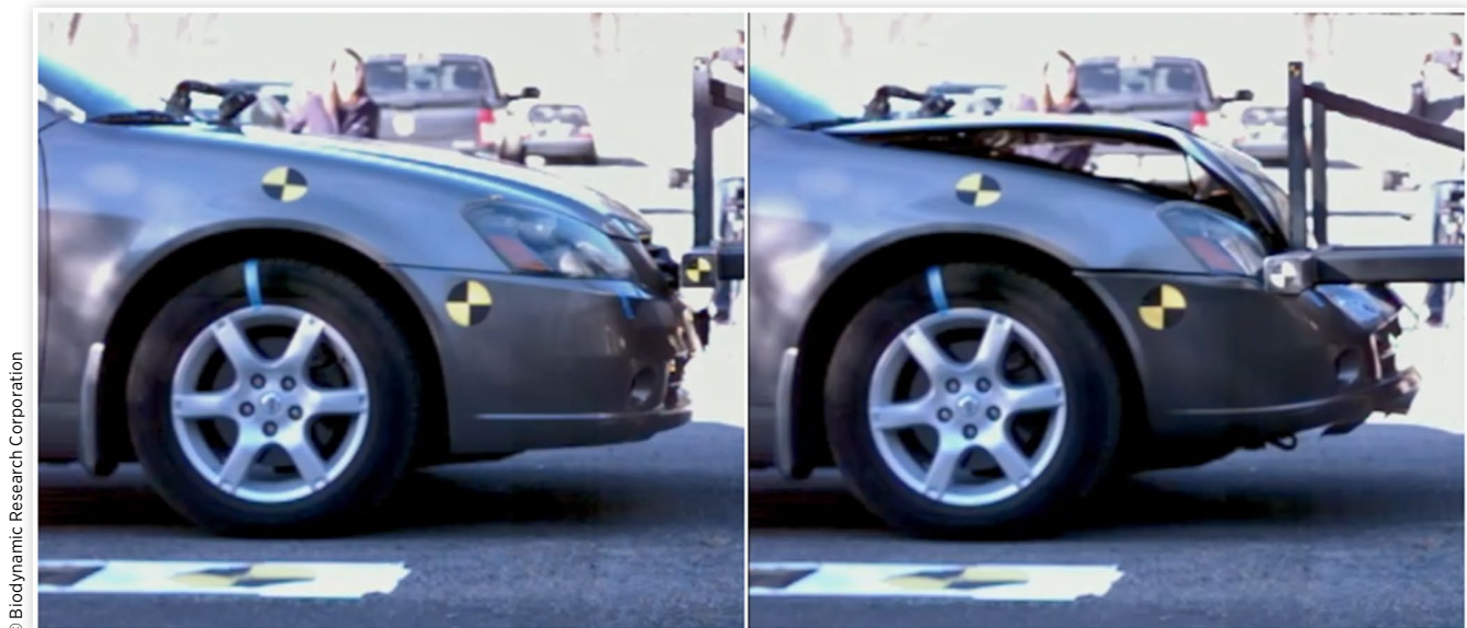
FIGURE 27 Video frames of crash test #5 show the Altima and underride guard at initial contact (left) and near maximum engagement (right).
