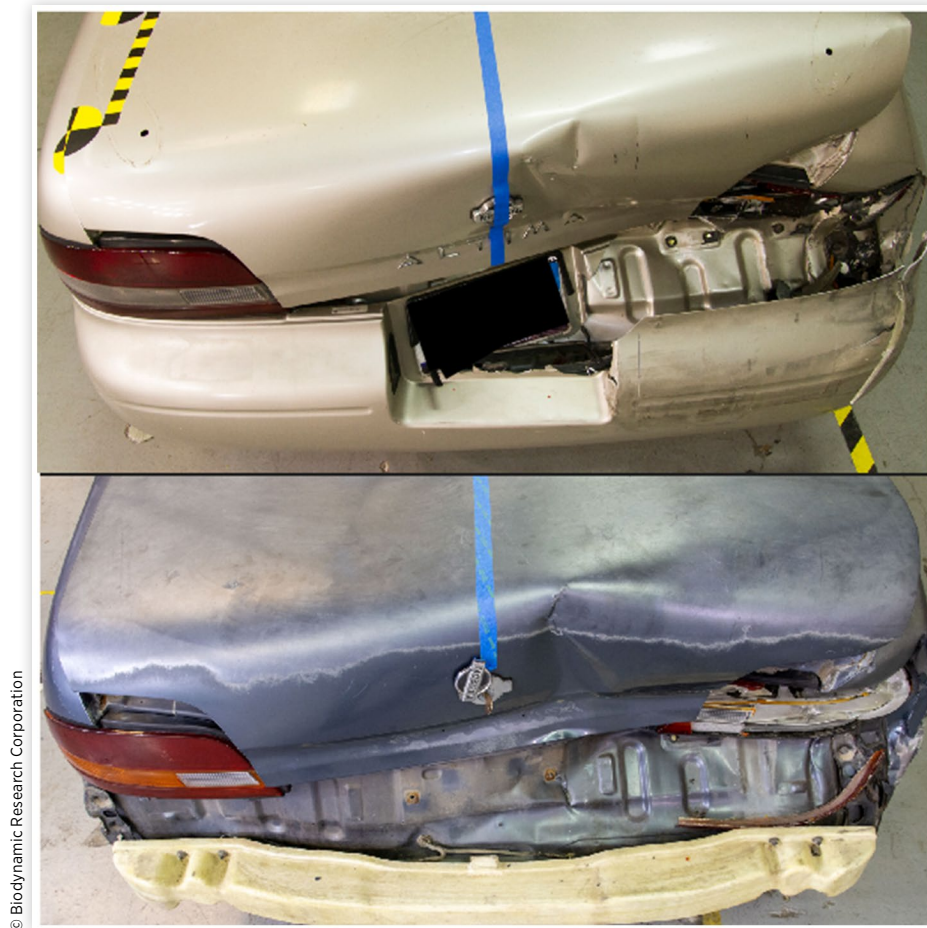
FIGURE 13 The top photograph shows the damage to the rear of the Altima in crash test #2, and the lower photograph shows the damage to the rear of the Altima as a result of the QSFJ measurement.
