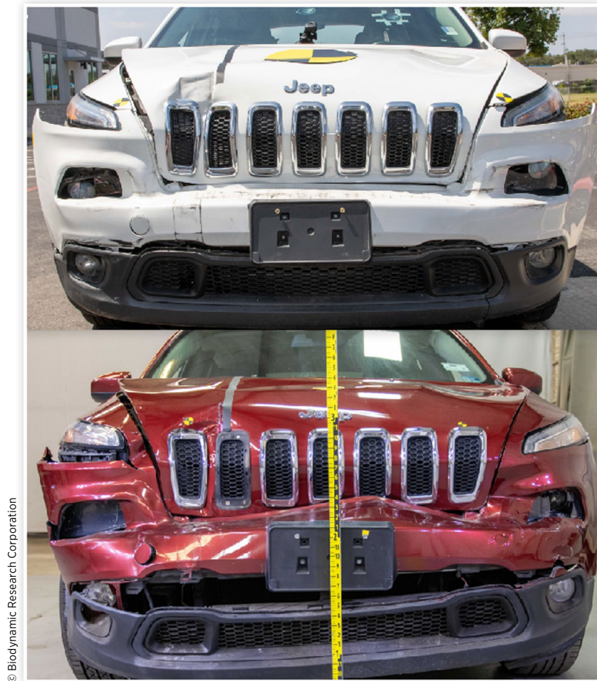
FIGURE 26 The top photograph shows the damage to the front of the Jeep Cherokee in crash test #4 and the bottom photograph shows the damage to the front of the Jeep used in the measurement of the QSFD data.
