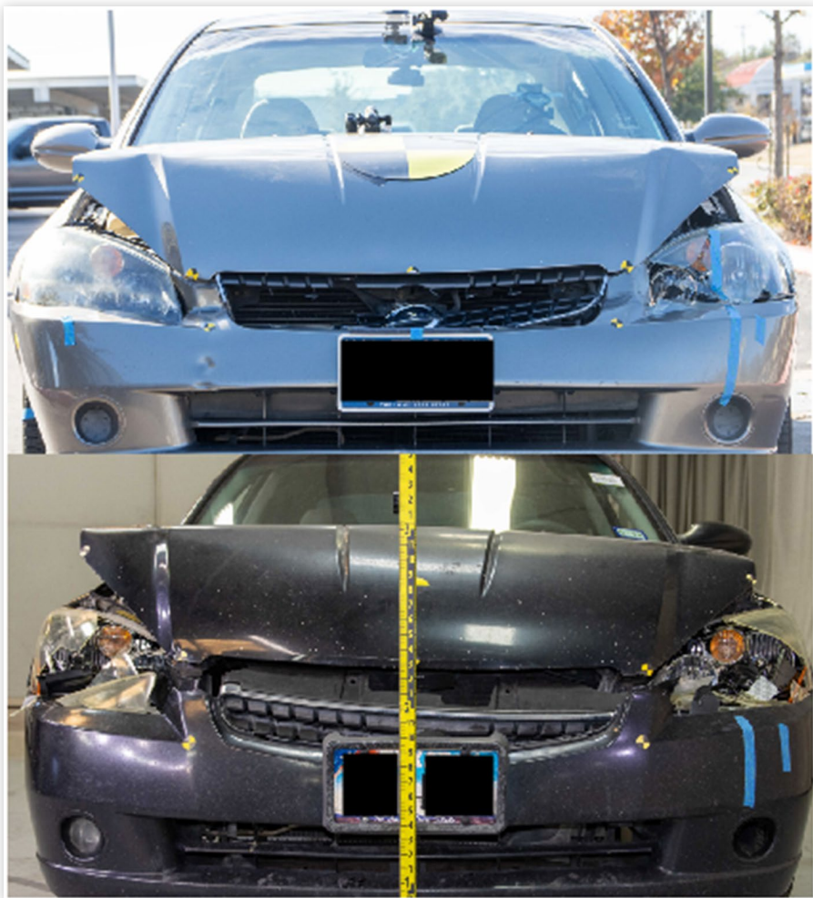
FIGURE 32 The top photograph shows the damage to the front of the Altima in crash test #5 and the lower photograph shows the damage to the front of the Altima used in the measurement of the QSF data.
