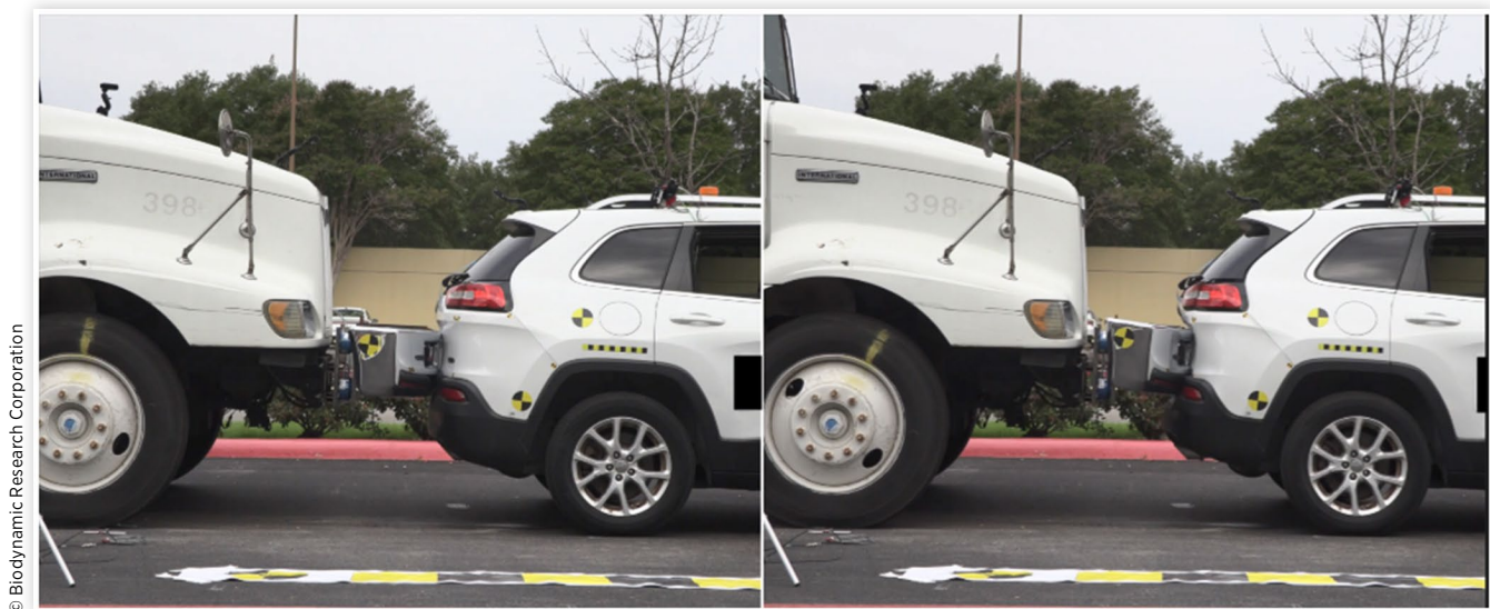
FIGURE 14 A lateral view of crash test #3 that shows the position of the vehicles at initial contact (left) and near maximum engagement (right).
