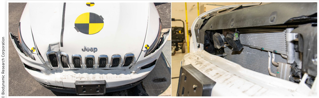
FIGURE 22 The damage to the front of the Jeep Cherokee in crash test #4.
