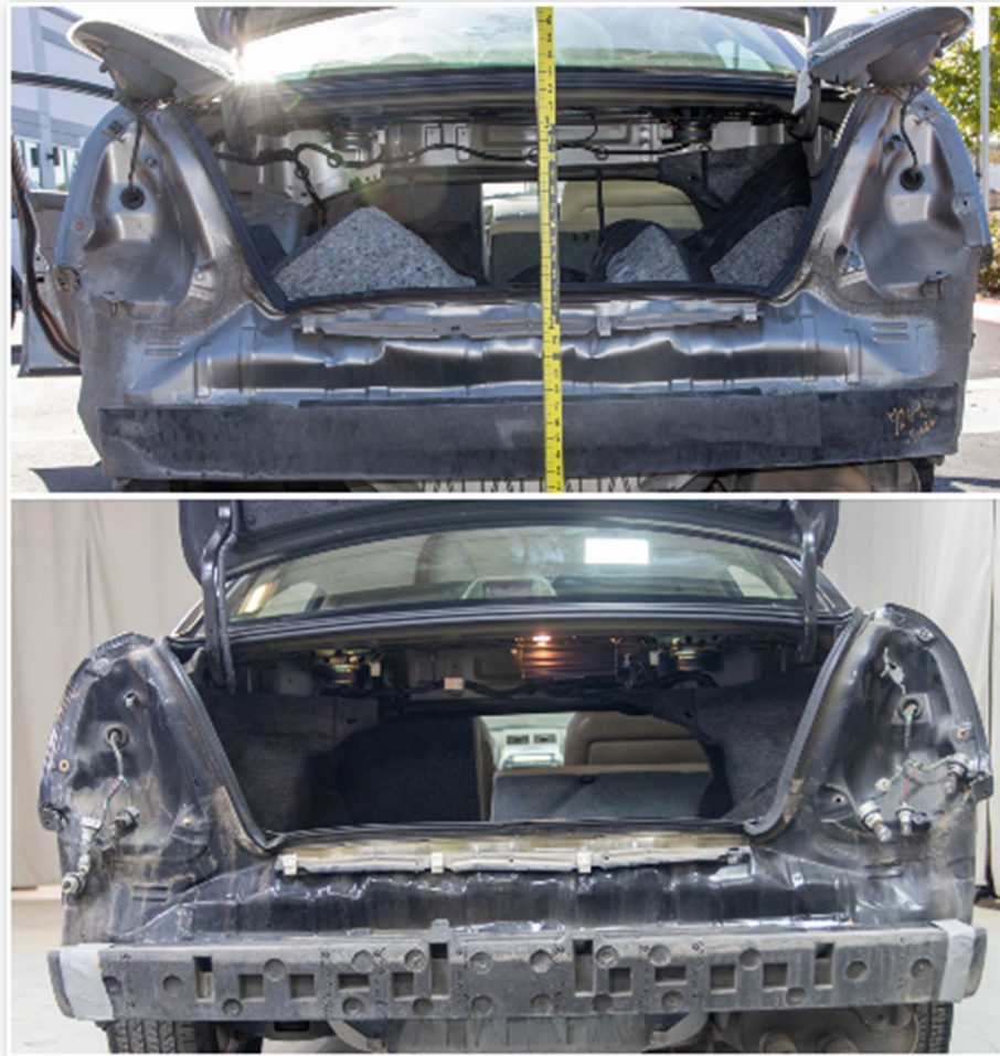
FIGURE 7 The top photograph shows the damage to the rear of the Altima in crash test #1 and the lower photograph shows the damage to the rear of the Altima used in the measurement of the QSFD data.
