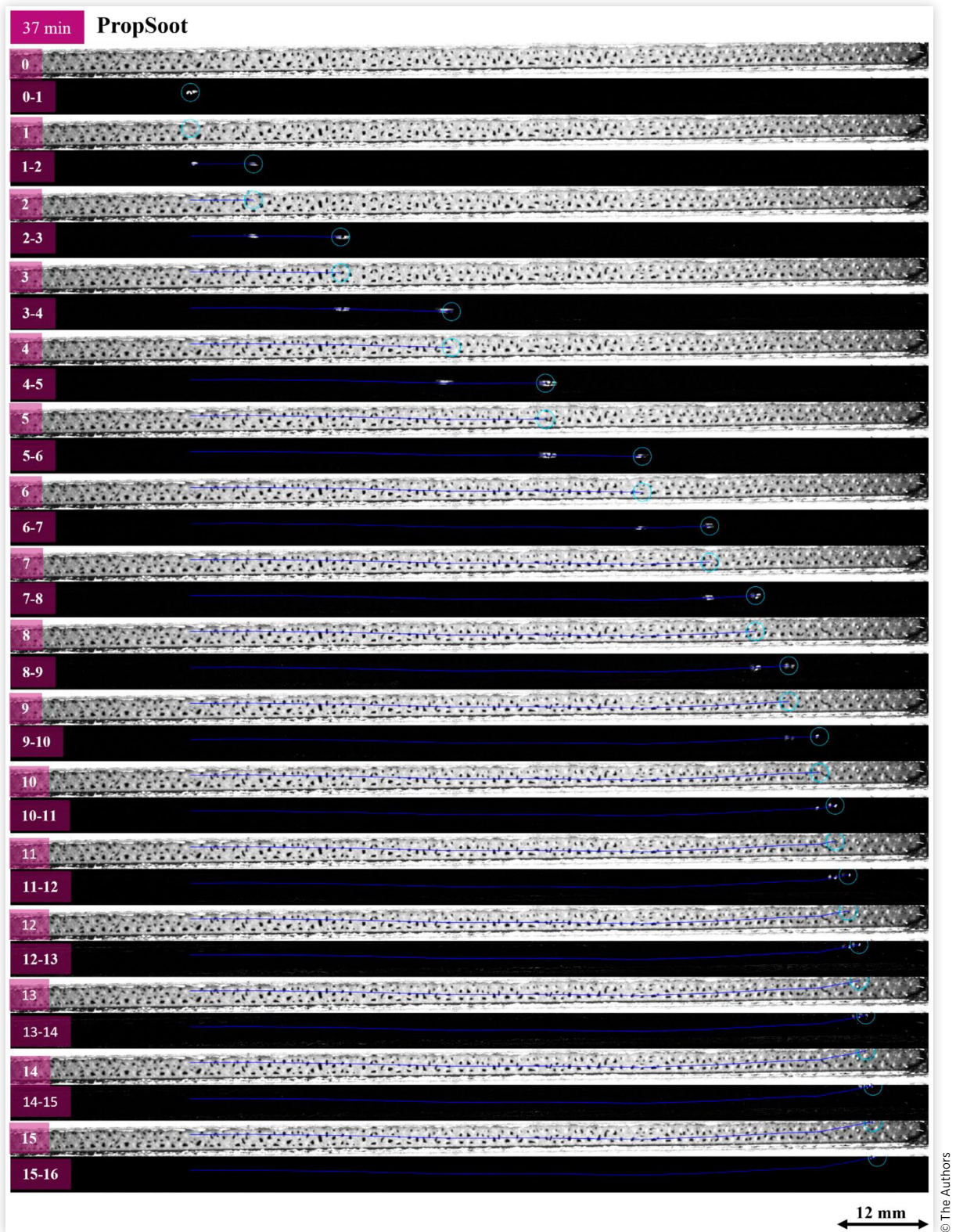
FIGURE 19 Representative image sequence of a PropSoot structures detaching and relocating at 37 min.
