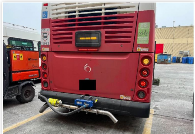
FIGURE 3 Rear of test vehicle, showing the exhaust flow meter attached to the tailpipe, along with heated sample lines for on-board instrumentation (Semtech LDV and AVL PM-PEMS).
