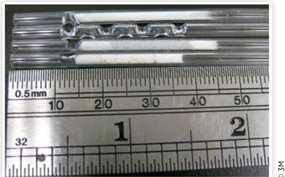
FIGURE 10 Illustration of cryo trap liners (from Gerstel CIS4) filled with glass wool, baffled empty, filled with glass beads, and filled with Tenax® TA (top to bottom).
