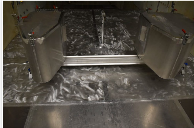
(a) Close-up showing water deflection plates
