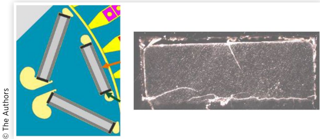
FIGURE 8 Cross-sectional geometry of a design variant with encapsulated magnets and result of first practical experimentation of magnet encapsulation [30].
