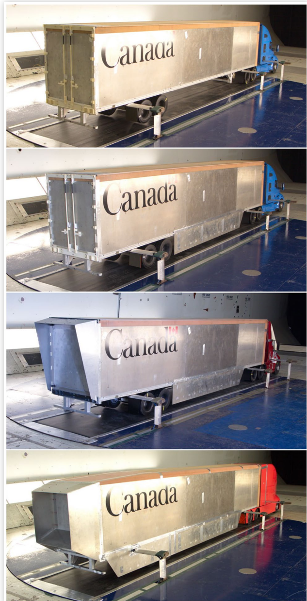
FIGURE 6 Photographs of tested dry-van-trailer configurations, top to bottom: standard; side skirts; side skirts and boat tail; low-drag trailer.
