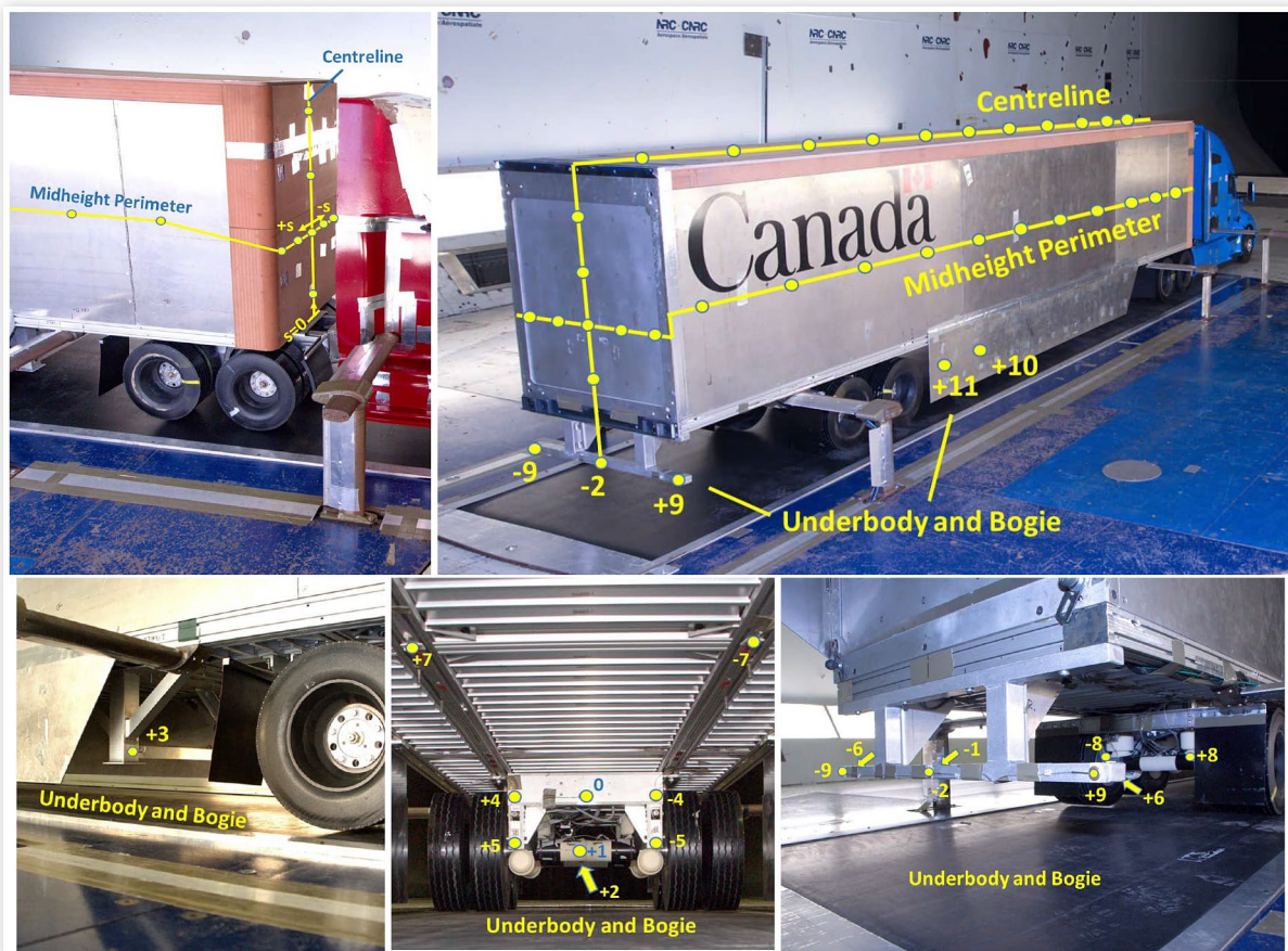
FIGURE 10 Pressure-tap locations for the dry-van-trailer model. Centreline and Midheight Perimeter tap locations are based on surface distance “ s ” with origins identified in upper left image.
