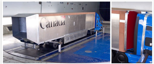
FIGURE 6 Low-drag trailer model with side-skirts, large boat-tail, trailer fairing, and single-wide tires with wheel covers. Front-face trailer fairing shown in red in the right photograph.
