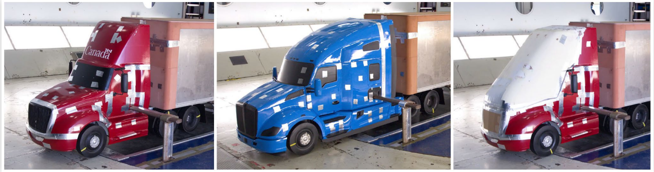
FIGURE 6 Low-drag trailer model with side-skirts, large boat-tail, trailer fairing, and single-wide tires with wheel covers. Front-face trailer fairing shown in red in the right photograph.
