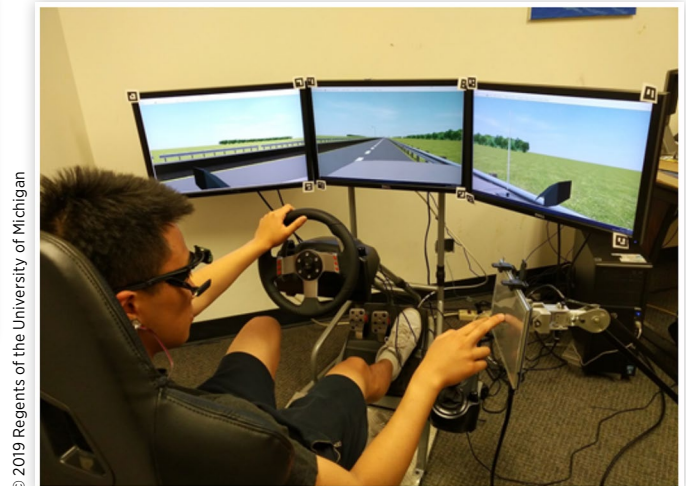
FIGURE 3 Driving simulator and secondary task setup. This setup increased the realism of the experimental tasks. Markers were placed on each monitor and the touchscreen to identify surfaces for eye tracking.
