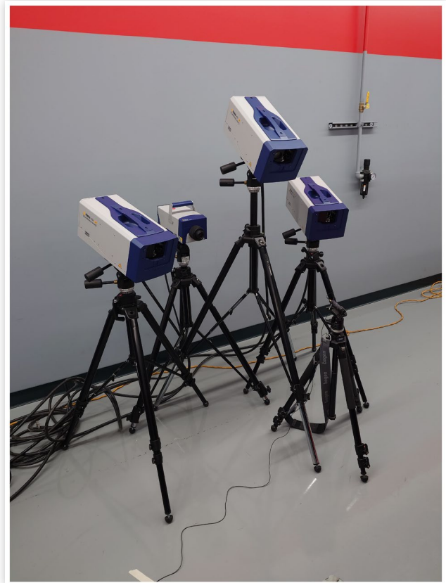
FIGURE 10 SLDV measurement setup in the chassis dynamometer environment for the rotating testing. The single-point reference laser is second from left. The laser tachometer is located at front on a short tripod.
