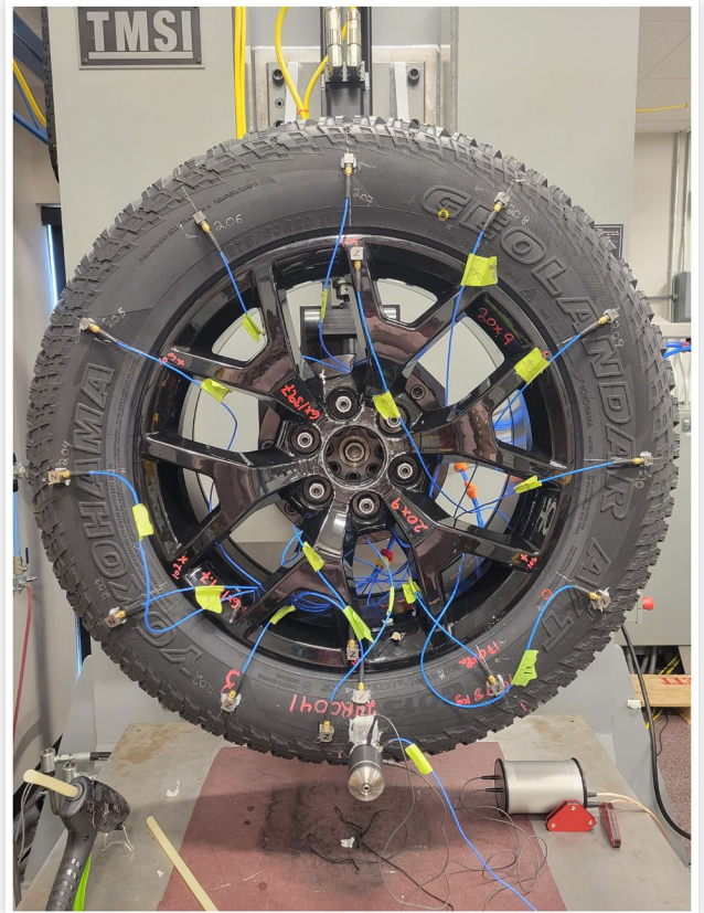
FIGURE 2 Fixed testing of the tire using accelerometers and an integral shaker. The tire is fixed at the wheel center in the laboratory. Note the clearance space between the bottom of the tire and the surface below. In the loaded testing, the tire is subjected to a vertical load, and it comes into contact with the surface below.
