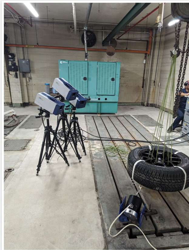
FIGURE 3 Free testing of the tire using the SLDV system and an electrodynamic shaker. The tire is suspended from bungee cords in the laboratory.
