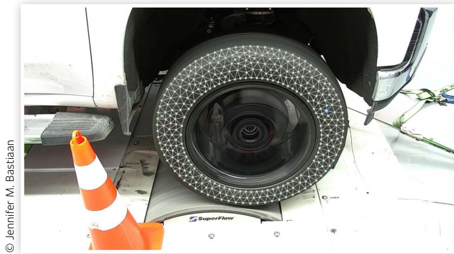
FIGURE 11 SLDV scan points in the chassis dynamometer environment for the rotating testing.
