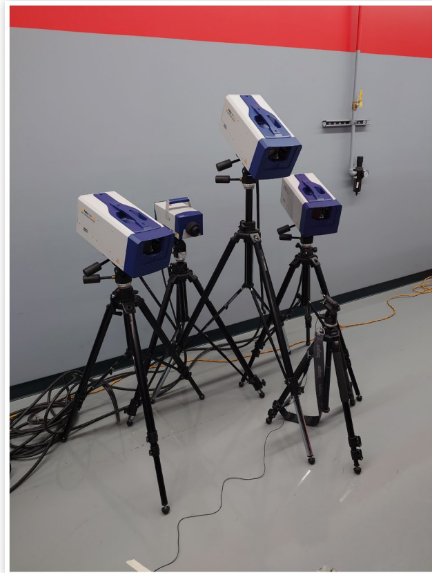
FIGURE 10 SLDV measurement setup in the chassis dynamometer environment for the rotating testing. The single-point reference laser is second from left. The laser tachometer is located at front on a short tripod.
