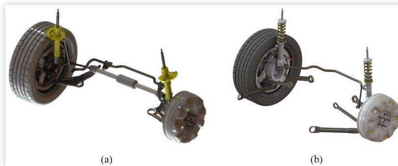
FIGURE 8 Vehicle corners with in-wheel motors on (a) front suspension and (b) rear suspension.
