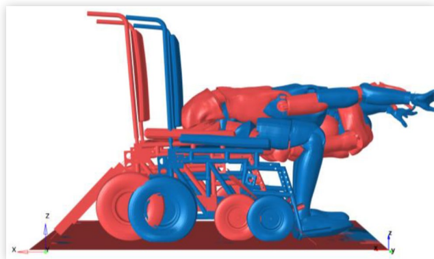
FIGURE 1 Comparison of excursions under frontal loading conditions for recommended (red) and vertical (blue) tiedown geometry at 180 ms.
