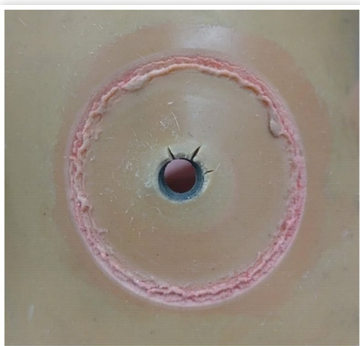
FIGURE 17 Clamping disk wear pattern on the membrane material after motored tests. (The pink hue is due to a red lubricant used between the membrane and disk to aid assembly and reduce friction during testing.)
