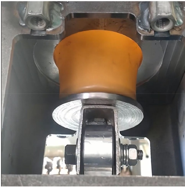
FIGURE 3 Stretched membrane in BDC position in the test bench.
