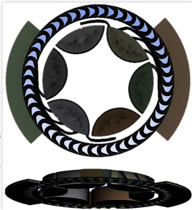
FIGURE 5 Simulation model of the hybrid concept of turboshaft engine (general and top view).
