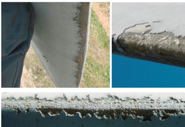
FIGURE 8 Leading edge erosion (LEE) of a wind turbine. Data taken from Ref. [29].
