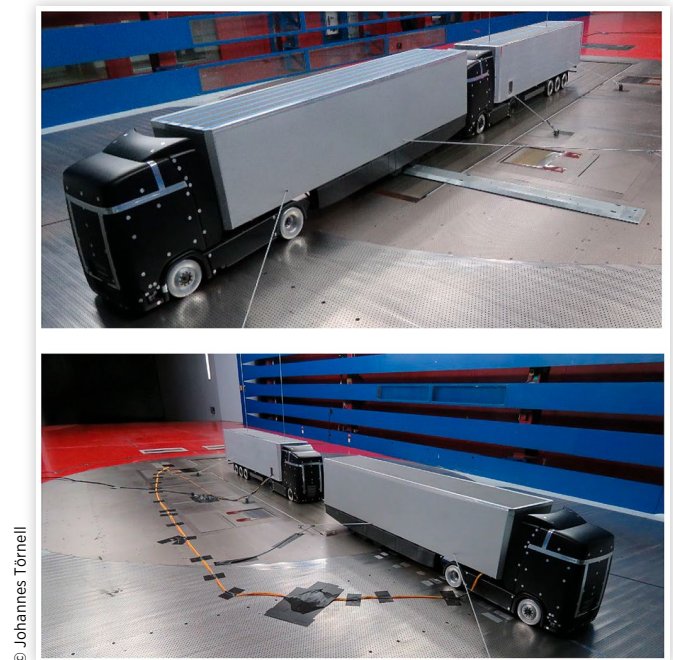
FIGURE 3 Mounting solution: leading truck is the dummy model and trailing truck is the measurement model. Top image is with the beam and bottom without.
