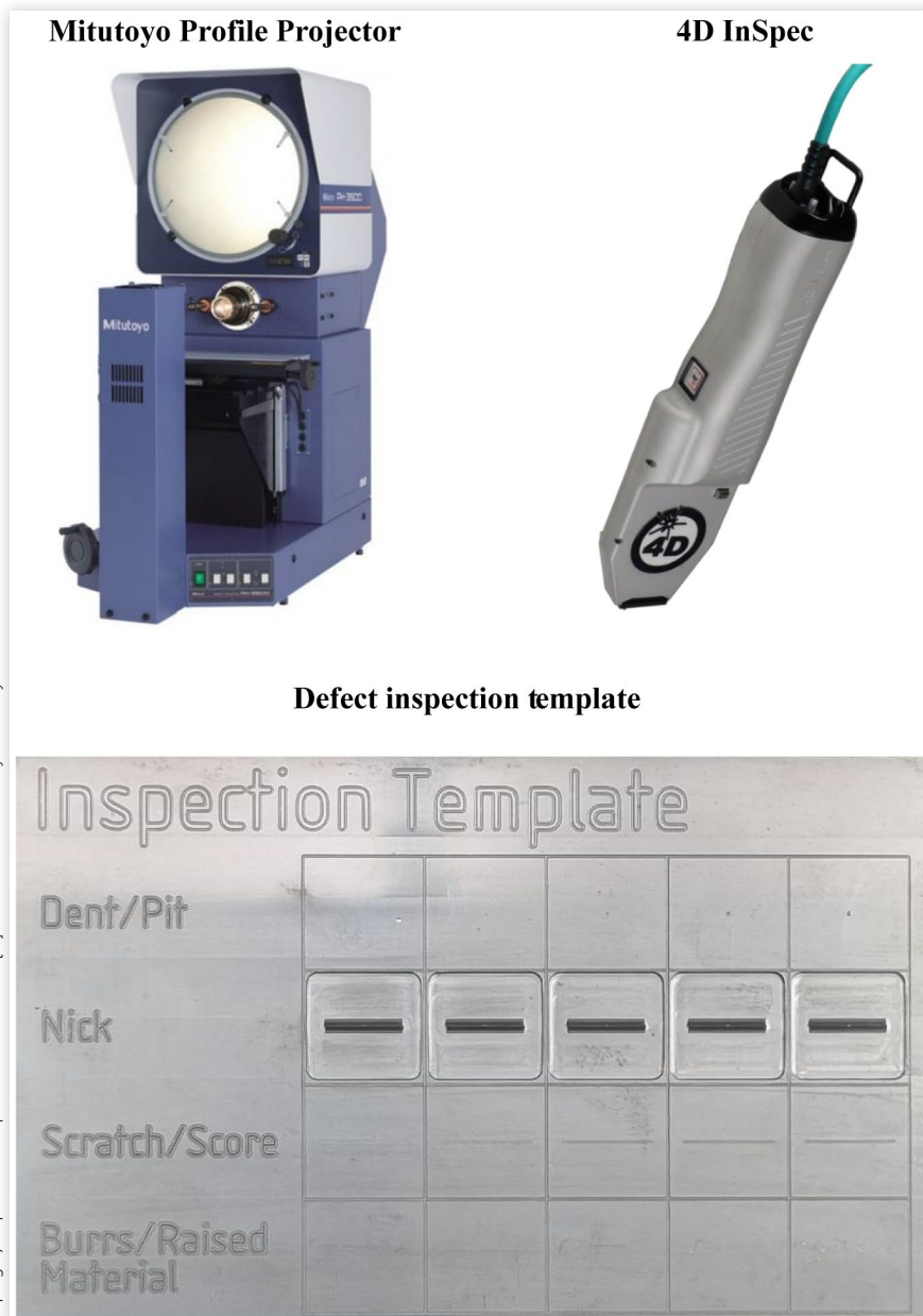
FIGURE 1 Overview of test equipment: Mitutoyo Profile Projector (top left); 4D InSpec Surface Gage (top right); Defect Inspection Template® (bottom).
